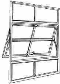
Fig. 4 Typical rolled steel windows available from 1890 to the present. The various operating and ventilating capacities in combination with the aesthetics of the window style were important considerations in the selection of one window type over another. Drawings: Sharon C. Park, AIA.
