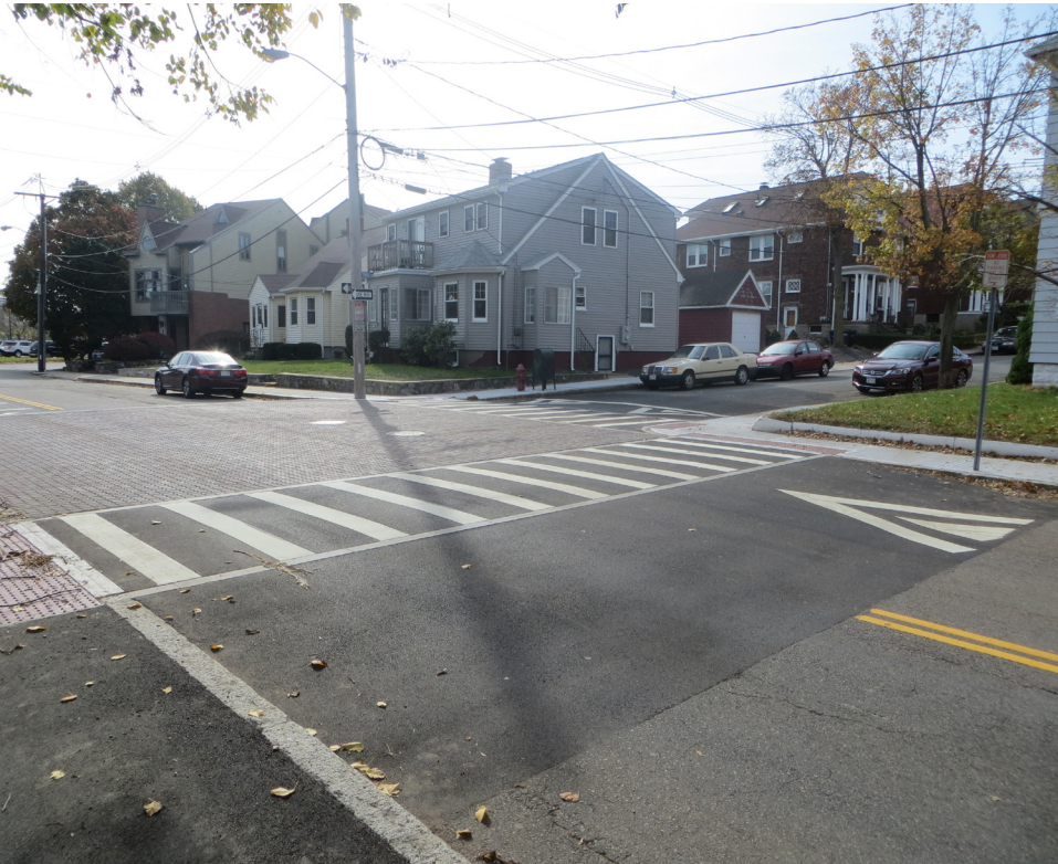
Example of a raised intersection with interlocking pavers in Somerville, MA
