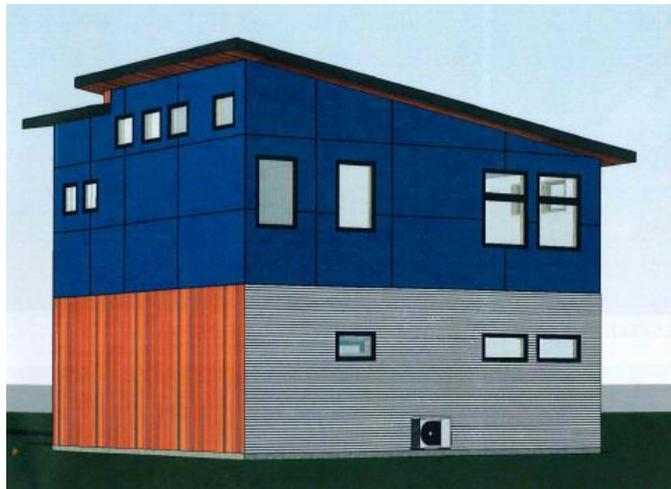
The design proposes Western Red Cedar on the first floor, and Fiber Cement Panels on the upper floor. A standing metal seam roof is identified on Plan A200. While all are considered durable building materials, they have little reference within the immediate neighborhood.
