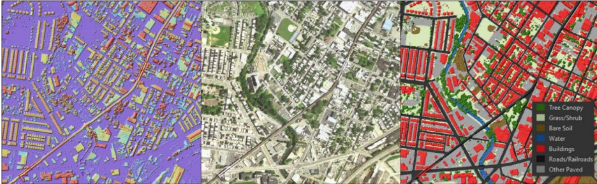
Figure 1A. High-resolution land cover products. Using LiDAR (left) and imagery (center) we derive high-resolution land cover (right), which provides a detailed and accurate accounting of a community's green, gray, brown, and blue infrastructure.
