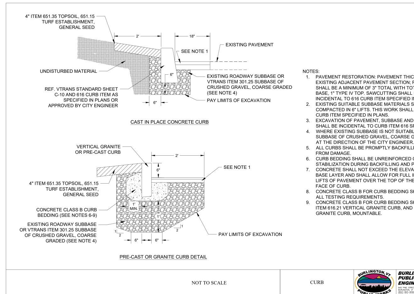
1. PAVEMENT RESTORATION: PAVEMENT THICKNESS SHALL MATCH EXISTING ADJACENT PAVEMENT SECTION: PAVEMENT THICKNESS SHALL BE A MINIMUM OF 3" TOTAL WITH TOTAL WIDTH 2" TYPE II BASE, 1" TYPE IV TOP, SAWCUTTING SHALL BE CONSIDERED INCIDENTAL TO 616 CURB ITEM SPECIFIED IN PLANS. 2. EXISTING SUITABLE SUBBASE MATERIALS SHALL BE REUSED AND COMPACTED IN 6" LIFTS. THIS WORK SHALL BE INCIDENTAL TO 616
